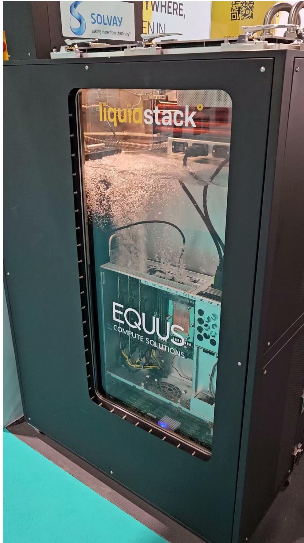
Liquid Stack, Liquid cool for data centers
